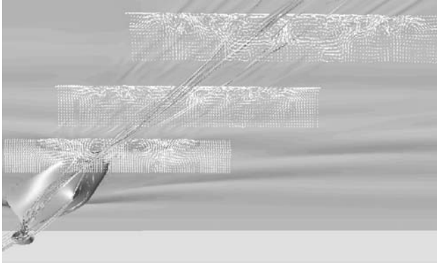
Figure 16.16. Surface ship flow: Perspective view of the stern of the DTMB 5415 hull at Fr = 0.28 , showing randomly released streamlines and three planes with secondary velocity vectors showing the vortical structures in the wake.
