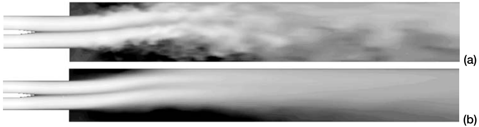
Figure 10.9. Plane sudden expansion: Contours of (a) axial velocity and (b) time-averaged axial velocity at the center plane of the ORACLES rig.
