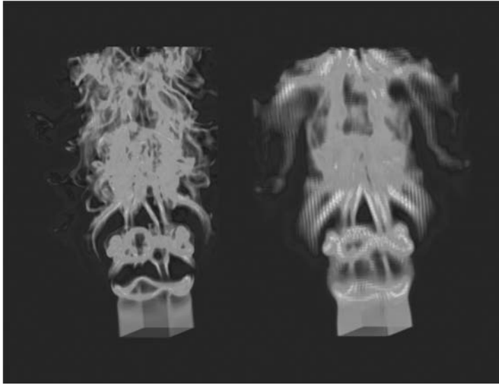
Figure 8.10. Comparative instantaneous volume visualization of the vorticity magnitude based on the database of square jets at the same time simulations on the finest grid left, and coarsest grid right (from Grinstein 2001). (See color inset, Plate 8).
