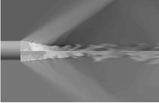
Figure 11.27. Density: The top half is without mass injection and the bottom half is with mass injection.
