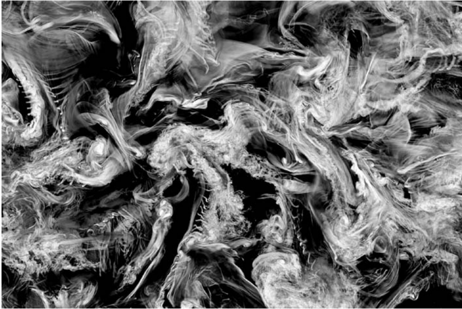
Figure 7.4. Volume rendering of a thin diagonal slice through the cube of turbulence computed at NCSA in 2003 with our PPM–Euler code on a grid of 2048^3 cells. The logarithm of the vorticity magnitude is shown. The flow is shown at 1.15 sound or flow-crossing times (the initial rms velocity is Mach 1) of the energy-containing scales, which are half the size of the cubical computational domain. At this stage it is clear that small-scale turbulence is developing more rapidly in some regions of this flow than in others, despite the statistical homogeneity imposed on the initial condition for the problem. Analysis of the flow on larger scales in these regions can reveal why the turbulence is developing rapidly there and not elsewhere. (See inset, Plate 3).
