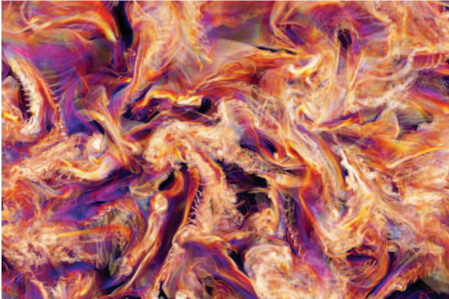
Plate 3. (Fig. 7.4) Volume rendering of a thin diagonal slice through the cube of turbulence computed at NCSA in 2003 with our PPM-Euler code on a grid of 2048^3 cells. The logarithm of the vorticity magnitude is shown. The flow is shown at 1.15 sound or flow-crossing times (the initial rms velocity is Mach 1) of the energy-containing scales, which are half the size of the cubical computational domain. At this stage it is clear that small-scale turbulence is developing more rapidly in some regions of this flow than in others, despite the statistical homogeneity imposed on the initial condition for the problem. Analysis of the flow on larger scales in these regions can reveal why the turbulence is developing rapidly there and not elsewhere.
