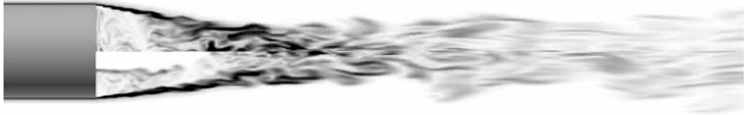
Figure 11.26. Vorticity: The top half is without mass injection and the bottom half is with mass injection.
