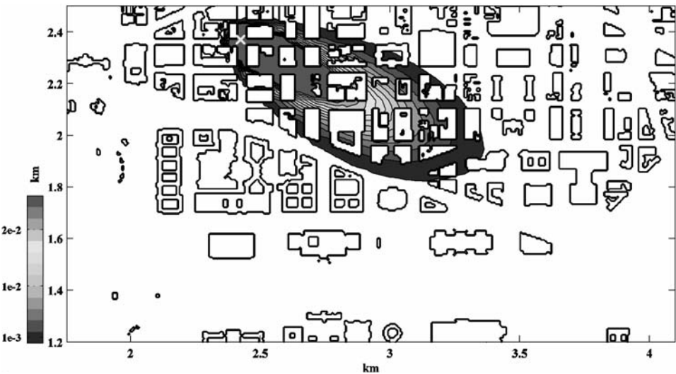
Figure 17.2. Washington DC dosage ( \text{kg s m}^{-3} ) after 12 min for the SCIPUFF Gaussian model prediction (Pullen et al. 2005).
